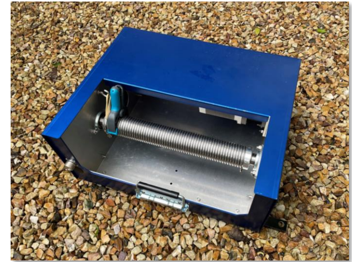
Portable electronically controlled winch
