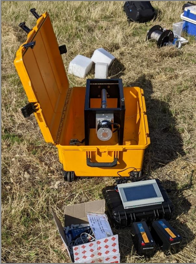
Customised electronic winch
