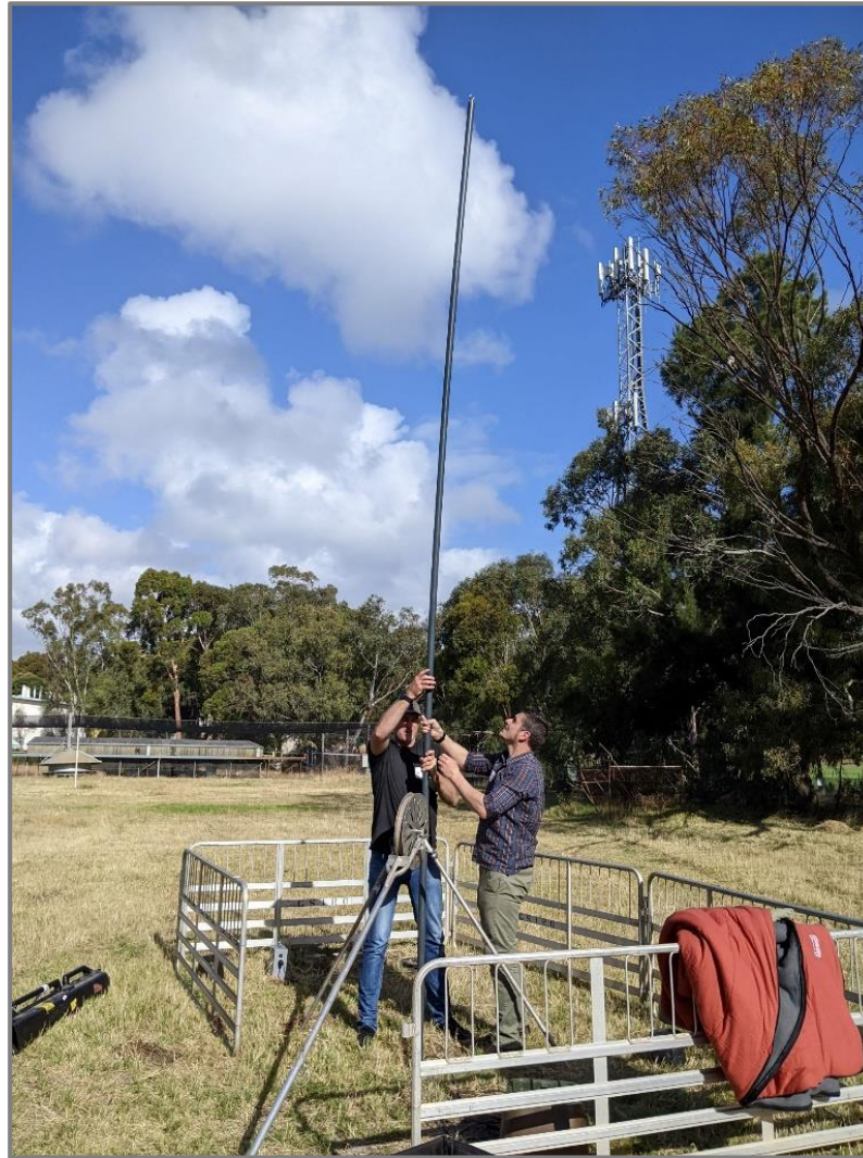
Extendable 6-metre-long PVC slug (40 mm OD)
