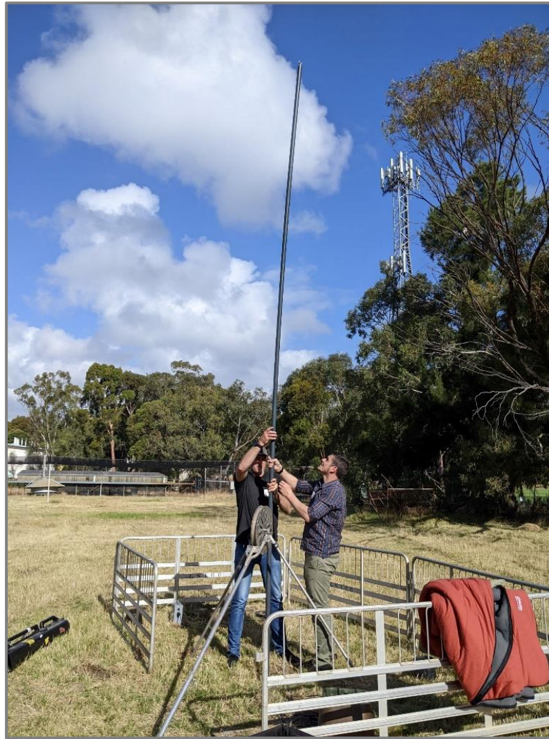
Extendable 6-metre-long PVC slug (40 mm OD)
