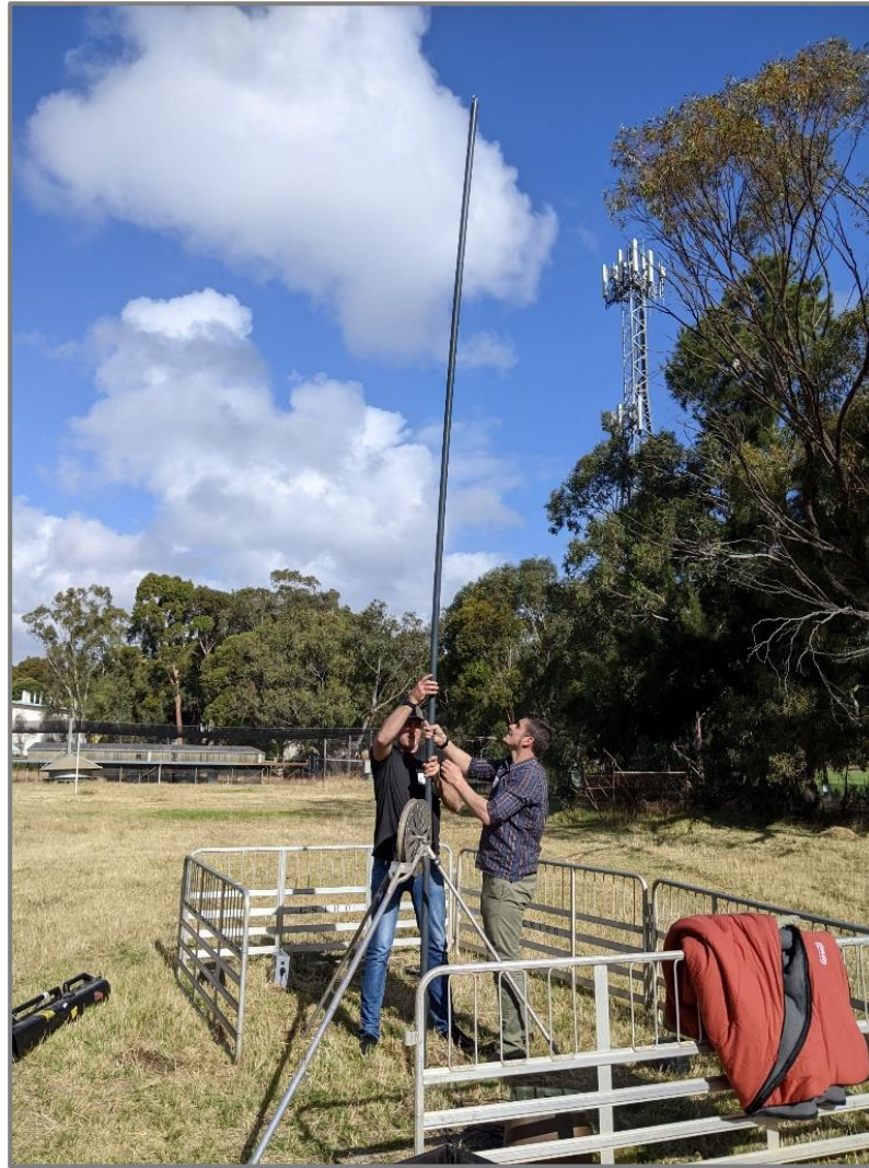
Extendable 6-metre-long PVC slug (40 mm OD)
