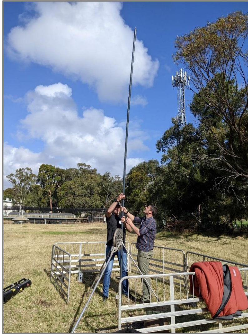
Extendable 6-metre-long PVC slug (40 mm OD)
