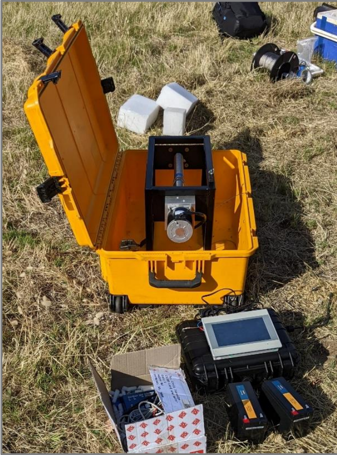
Customised electronic winch
