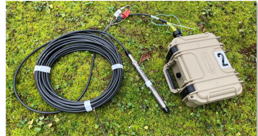
Wireless observation well node, including sensor and cable
