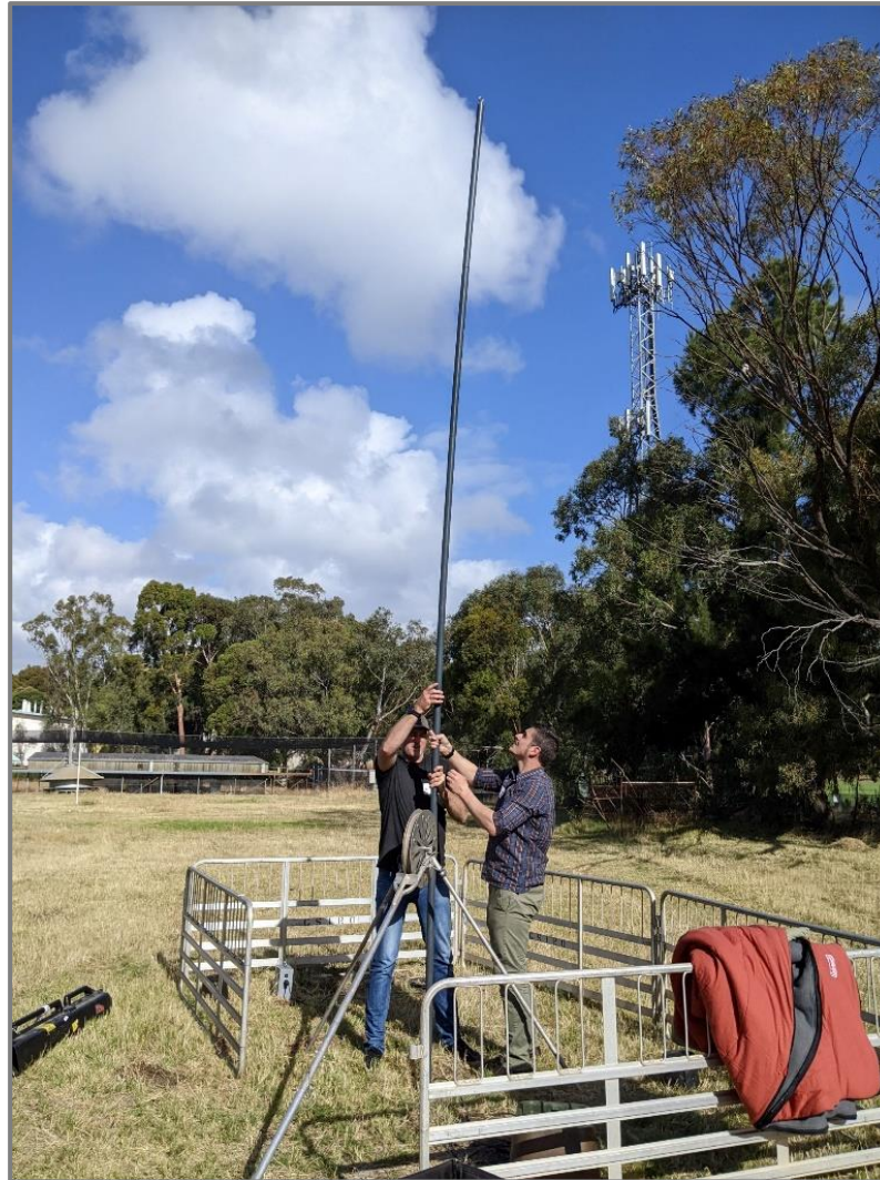
Extendable 6-metre-long PVC slug (40 mm OD)
